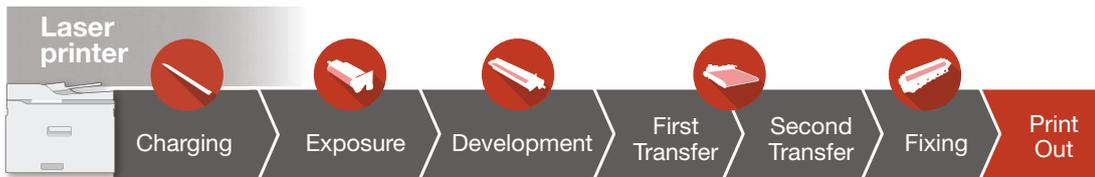
Complex technology using **heat** and **pressure**
