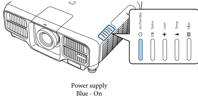
When the projector is in standby status, remove the USB flash drive.
