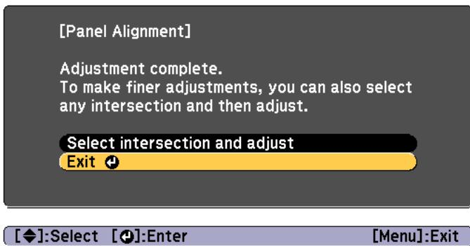
If you feel you still need to make adjustments after correcting all four points, select **Select intersection and adjust** and then continue making adjustments.
