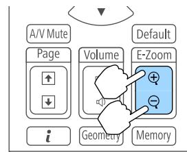
[+] button: Expands the area each time it is pressed. You can expand quickly by holding the button down.
