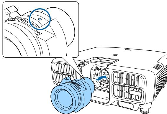
**4** While holding the lens unit firmly, hold the lock lever and turn it clockwise to lock the lens unit.
