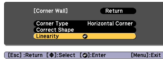
**13** Press the [ $\blacktriangleleft$ ][ $\triangleright$ ] buttons to adjust the linearity.
