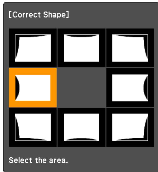
When selecting a corner, you can adjust the two sides next to the corner.
