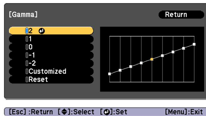
When a larger value is selected, the dark areas of images become brighter, but the color saturation for lighter areas may become weaker. When a smaller value is selected, you can reduce the overall brightness of the image to make the image sharper.
