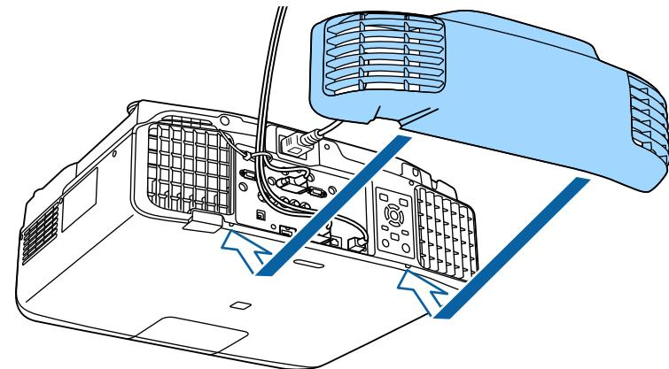
**3** Tighten the two screws on the cable cover. (You can tighten the screws with your fingers.)
