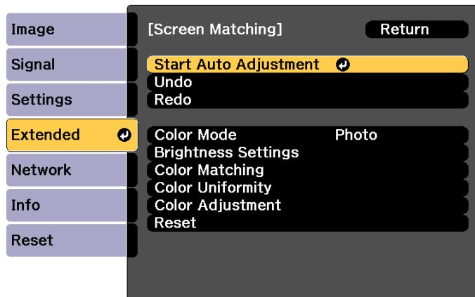
The adjustment pattern is displayed, and adjustment starts. If the projected image is displayed before the adjusting, the procedure is complete.
