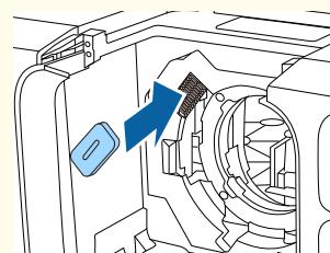
**3** Insert the lens unit straight into the lens insertion section with the white circle on the lens on top.
