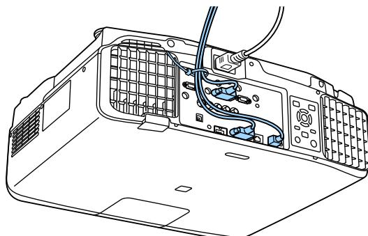
**2** Insert the tabs on the cable cover into the two slots on the back of the projector.
