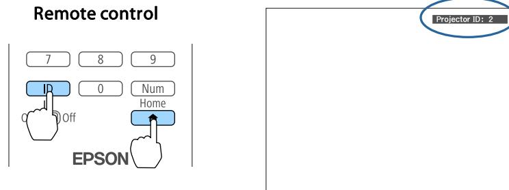
When you press the buttons, the current Projector ID is displayed on the projection screen. It disappears in about three seconds.
