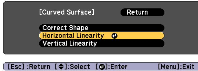
Select **Horizontal Linearity** to adjust the horizontal expansion or contraction, and select **Vertical Linearity** to adjust the vertical expansion or contraction.
