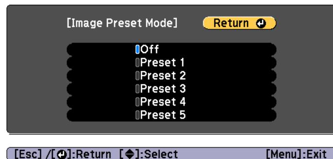
After selecting **Preset 1** to **Preset 5**, you can fine tune each setting individually. The setting after adjustment will be overwritten.
