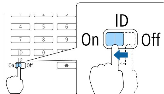
**2** While holding the [ID] button, press a number button to select a number to match the ID of the projector you want to operate.
