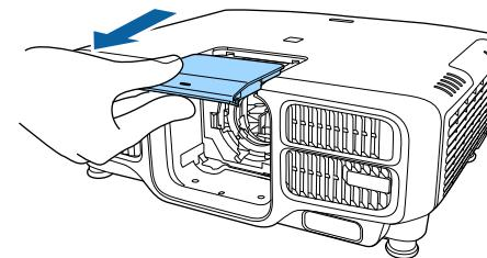
**2** Hold the lock lever and turn it counterclockwise.
