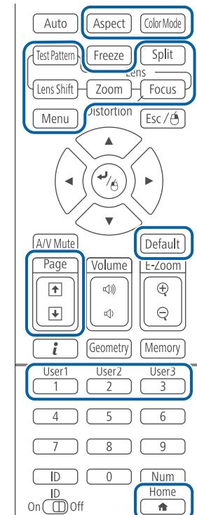
Each time the [
