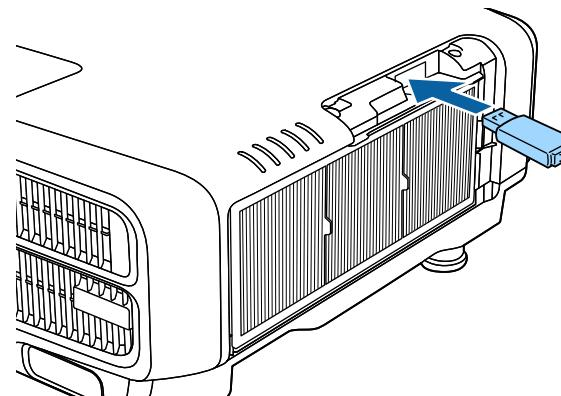
**4** When "Network information update complete. Remove the Quick Wireless Connection USB Key Adapter." is displayed, remove the Quick Wireless Connection USB Key Adapter.
