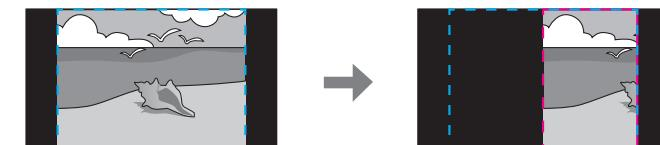
**Full Display**: Adjusts according to the projector's panel size (the maximum area in which an image can be displayed).
