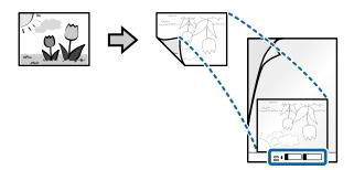
5. Load the Carrier Sheet with its leading edge directed to the ADF.
