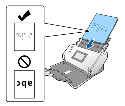
7. Adjust the edge guides to fit the originals without any gap. Otherwise, the originals may be fed skewed.
