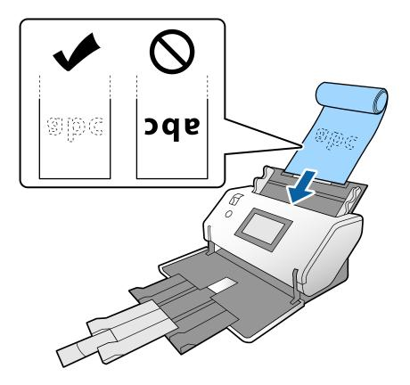
5. Adjust the edge guides to fit the original without any gap. Otherwise, the original may be fed skewed.
