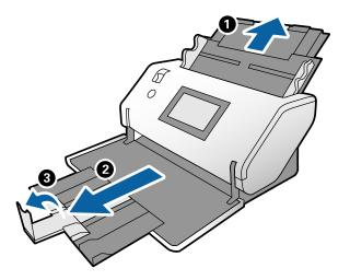
$^{3}\cdot$  While holding the tab, slide the edge guides all the way out.
