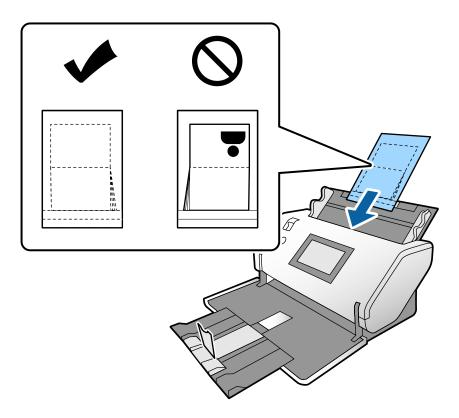
6. Adjust the edge guides to fit the Passport Carrier Sheet without any gap.
