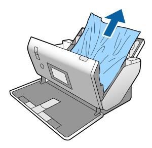
4. If you cannot pull originals straight up, carefully pull out any jammed originals from the output tray in the direction of the arrow.
