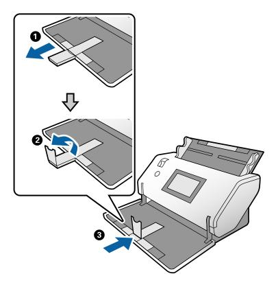
3. While holding the tab, slide the edge guides all the way out.
