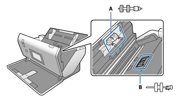
A: Separation Roller, B: Pickup Roller
