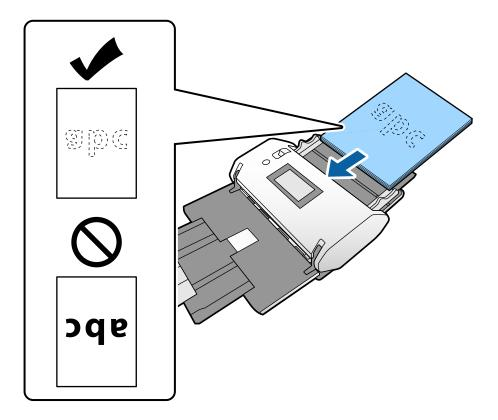
8. Adjust the edge guides to fit the original without any gap. Otherwise, the original may be fed skewed.
