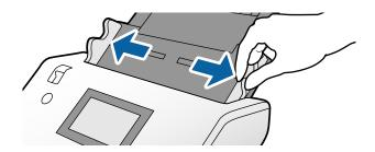
4. Load the booklet into the input tray with the printed surface facing down, and the thicker side aligned with the leading edge line, as shown in the diagram.
