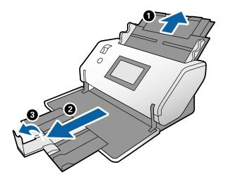
3. While holding the tab, slide the edge guides all the way out.
