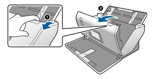
5. Open the cover of the Pickup Roller, and then slide and remove it.
