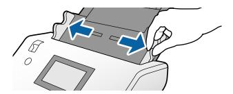
4. Load the cards with the side to be scanned facing down and their leading edge directed to the ADF.
