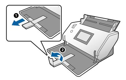
3. While holding the tab, slide the edge guides all the way out.
