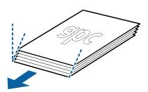
7. Load the originals with the side to be scanned facing down and the leading edge directed to the ADF. Insert the paper into the ADF until it meets resistance.
