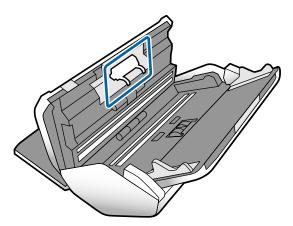
${\it \$}. \quad \hbox{Wipe off any dust or dirt on the Separation Roller using a genuine Epson cleaning kit or a soft, moist cloth.}$
