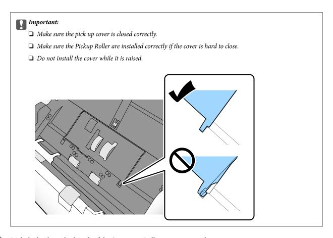
. Push the hooks on both ends of the Separation Roller cover to open the cover.
