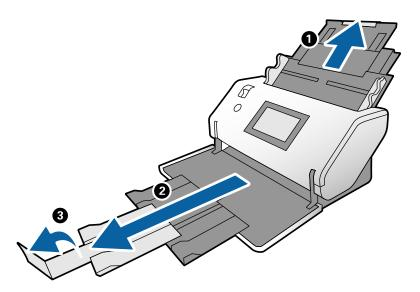
3. While holding the tab, slide the edge guides all the way out.
