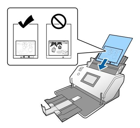
6. Align the edge guides with the Carrier Sheet without any gap. Otherwise, the Carrier Sheet may be fed skewed.
