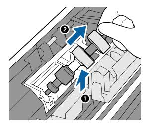
11. Insert the new separation roller axis into the hole, and then lower the roller.
