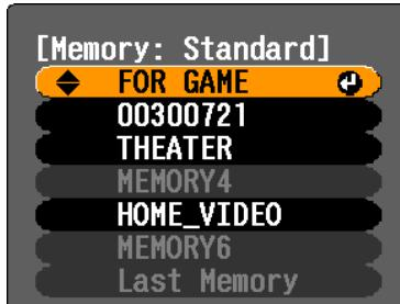
The adjustment results for all of the configuration menu items shown at left and the aspect setting can be saved. The "Memory: Standard" command in the "Image" menu is used to save the settings.
