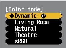
Press **▲** or **▼** on the remote control or **▲** or **▼** on the projector's control panel to select an item.
