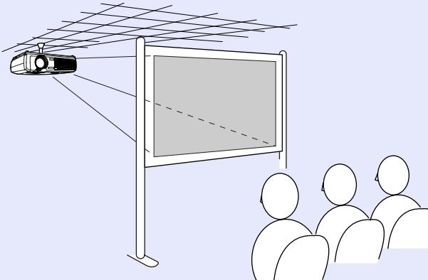
\* A special method of installation is required for suspending the projector from the ceiling. Please contact your supplier if you would like to use this installation method. The optional ceiling mount is required when installing the projector on the ceiling.
