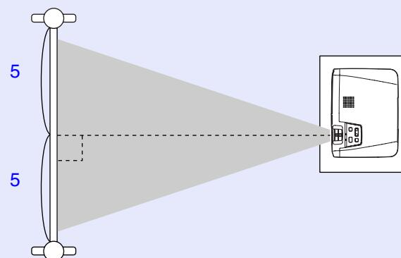
If it is not possible to set up the projector so that it is perpendicular to the screen, it can be set up at a slight vertical angle instead. You can extend or retract the front adjustable feet to adjust the upward projection angle within a maximum range of 10°.
