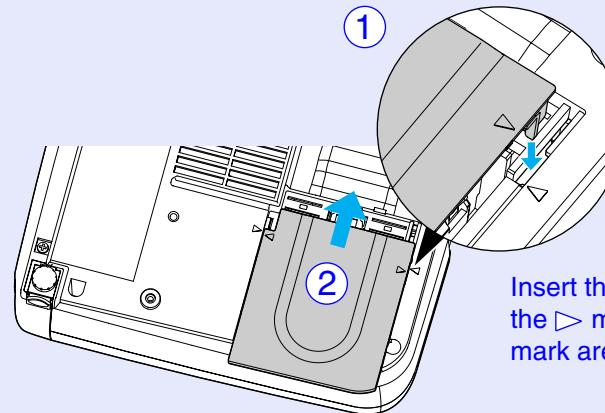
Insert the cover so that the ▷ mark and the < mark are aligned.
