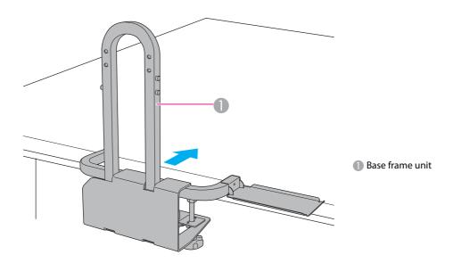
(3) Align one side of the U-shaped arch on the base frame unit ( 1) in the following illustration) and the supposed central line of the screen during projection ( 2) in the following illustration) to align the center of the lens and the center of the screen.
