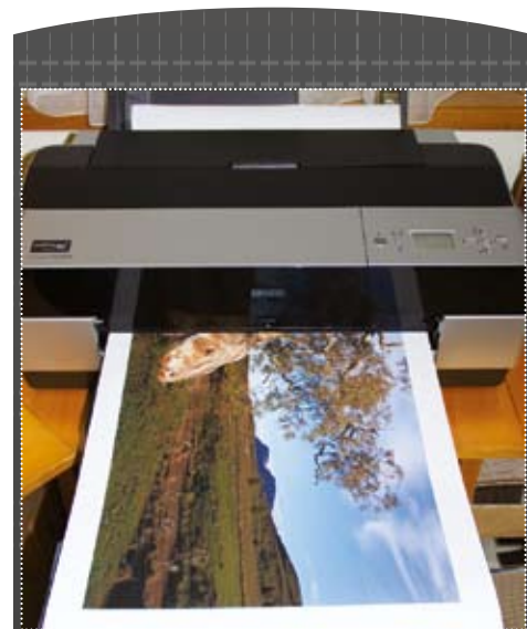
▲ A print made on the maximum paper size of 431.8x950 mm shown half-way through from the rear manual feeder.
