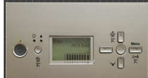
▲ A monochrome LCD read-out is provided on the 3880’s top deck and includes a set of ink level indicators.
