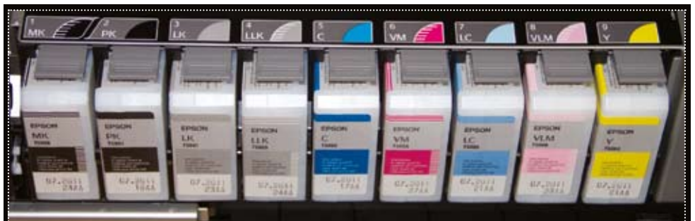
▲ The set of nine UltraChromeK3 pigmented inks. The Photo Black and Matte Black cartridges have their own individual slots.
