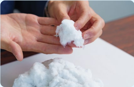
Innovative: Dry Fibre Technology can transform defibrated raw materials and process it into shapes according to the application.
