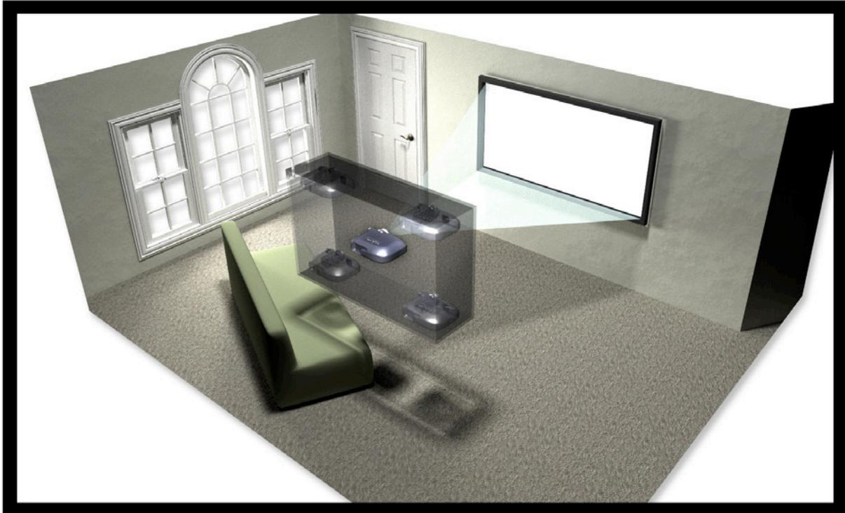
**Figure 4: A gray box shows the typical area a projector with lens shift could be moved to while still projecting the image onscreen.**
