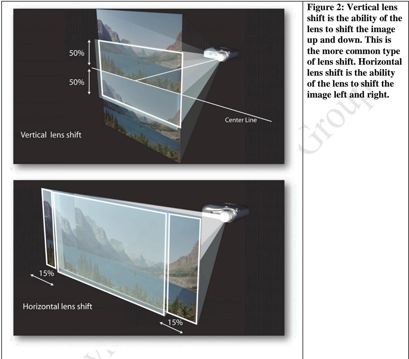
**Figure 2: Vertical lens shift is the ability of the lens to shift the image up and down. This is the more common type of lens shift. Horizontal lens shift is the ability of the lens to shift the image left and right.**
